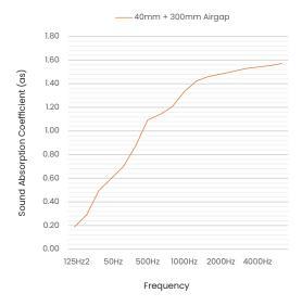
Weighted Sound Absorption Coefficient (aw) - Measured in accordance with ISO 11654. Practical sound absorption coefficient ap values at given standard frequencies are compared with reference curve aw.
