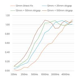
Weighted Sound Absorption Coefficient (aw) - Measured in accordance with ISO 11654. Practical sound absorption coefficient ap values at given standard frequencies are compared with reference curve aw.
